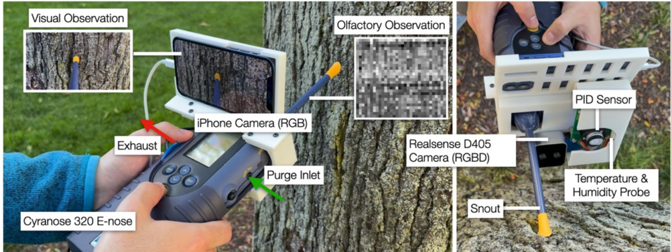
Figure 4. Capturing paired sight and olfaction. We walk through a variety of real-world scenes and capture paired olfaction and visual signals using a camera mounted to an e-nose on a custom 3D-printed sensor rig. We point the e-nose’s snout at each object or substance of interest and record multiple images and smell signals from different orientations. We also capture a suite of other supplementary modalities: depth (from an RGB-D camera), temperature, humidity, and ambient VOC concentrations (from a PID sensor).
